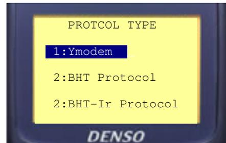
**Important** Once the new program has been loaded, the protocol must be set back to **BHT PROTOCOL** in order for the day to day data transfers to work correctly.
