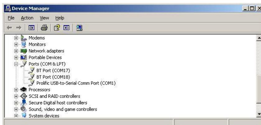
USB Active Port Connection. If using a USB cradle then check the virtual com port number in the system properties. To find this from the **Control Panel**, select **System** then select the **Hardware** tab then **Device Manager**. (For Windows 7 Select **Device Manager** from the **Control Panel**)
