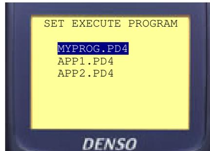
Ensure the loaded program is highlighted then press **ENT** now switch the unit off press **PW**.
